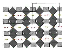
Framework Tetragonal Structure built up from [PO<sub>4</sub>] tetrahedra and [VO<sub>4</sub>F<sub>2</sub>] bi-octahedra with bridging Fluorine.
