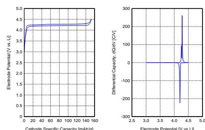
Theoretical Capacity - 155 mAh/g Reversible Specific Capacity!!
